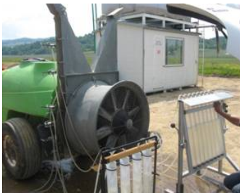
Figure 1. Measuring the capacity of the nozzle
